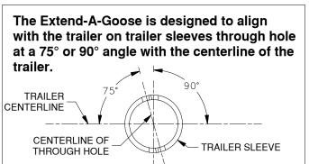
The centerline of the Extend-A-Goose coupler must be installed in line with the direction of travel. Failure to install the coupler properly could result in serious injury or death.
