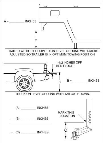
FIGURE A2: Trailer sleeve hole orientation.
