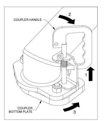
FIGURE B1: Coupler in "open" position
