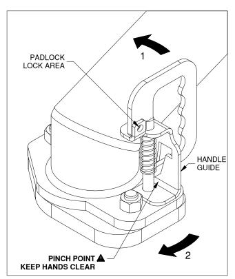
FIGURE B2: Coupler in "closed" position
